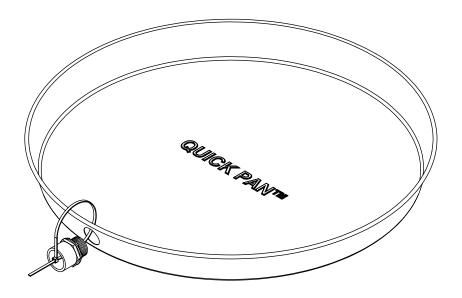
The HOLDRITE® QUICK PAN™ provides a quick simple solution when a drain pan is required under a water heater. These pans are suitable for both electric and gas water heaters. Available in six sizes (20" - 30"). Model #QP-20 (20"), #QP-22 (22"), #QP-24 (24"), #QP-26 (26"), #QP-28 (28") and #QP-30 (30"). Pan depth is 2-1/2".
